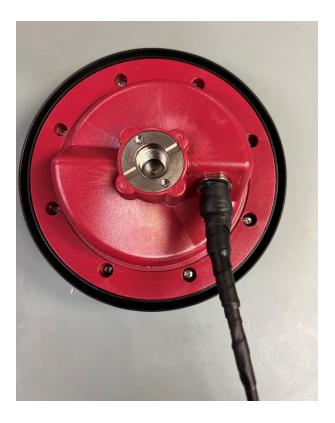
• Cover as much of the connector as possible. Stretch the tape into the threads above the connector
