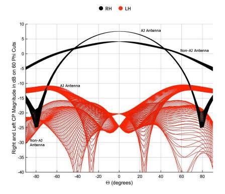
Radiation Pattern Comparison of an AJ antenna versus a Non-AJ antenna @1575MHz
