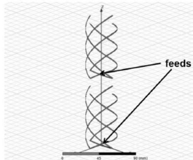
Figure 2. Two element quadrifilar helix array
