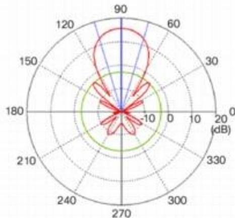
(c) Yagi Antenna Azimuth Plane Pattern
